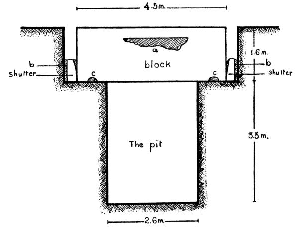
FIG. 10.-Transverse section showing the positions of gypsum mortar in a, b and c.
