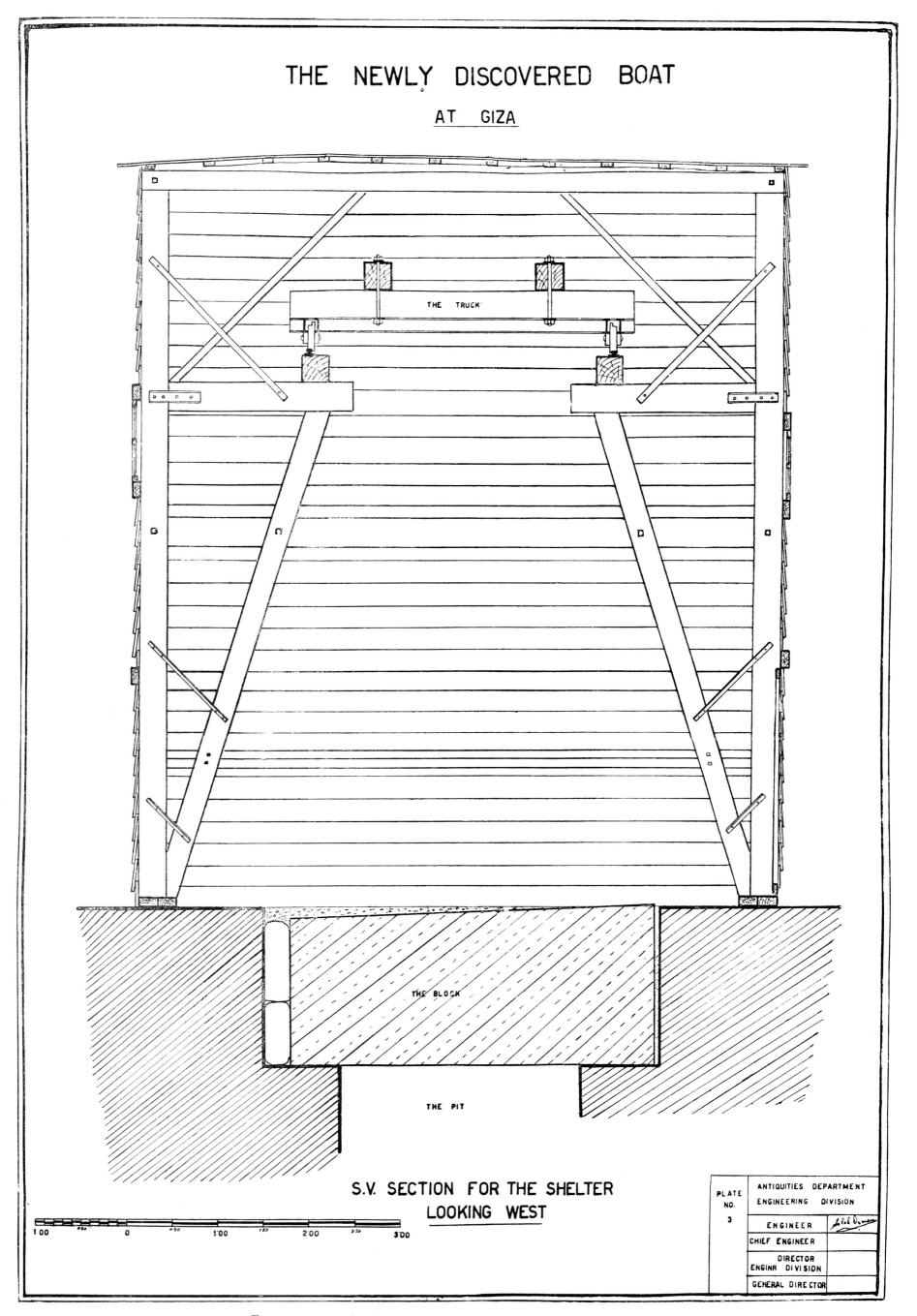
Transverse cross section of the shelter, showing the construction of the dolly truck.
