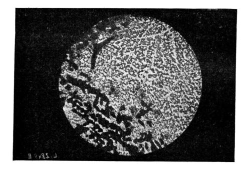
Fig. 17.—Microphoto of the previous staple showing details after treatment with copper chloride solution 88  $\times$ .
