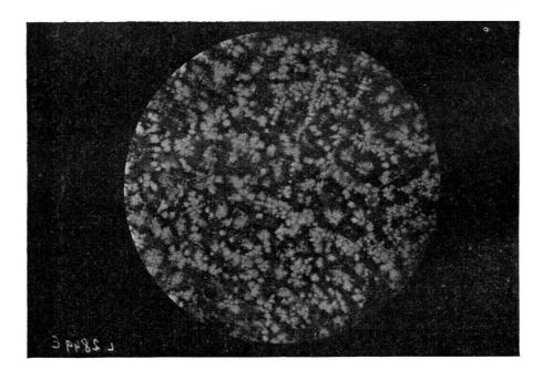
Fig. 18.-Microphoto of the previous staple, attacked by copper chloride solution: 259x.
