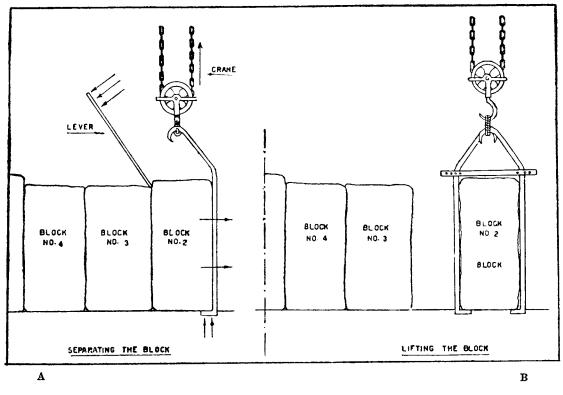
FIG. 9.—(A) Process of separating the block from the one next to it.(B) The use of the pickers in lifting the block.
