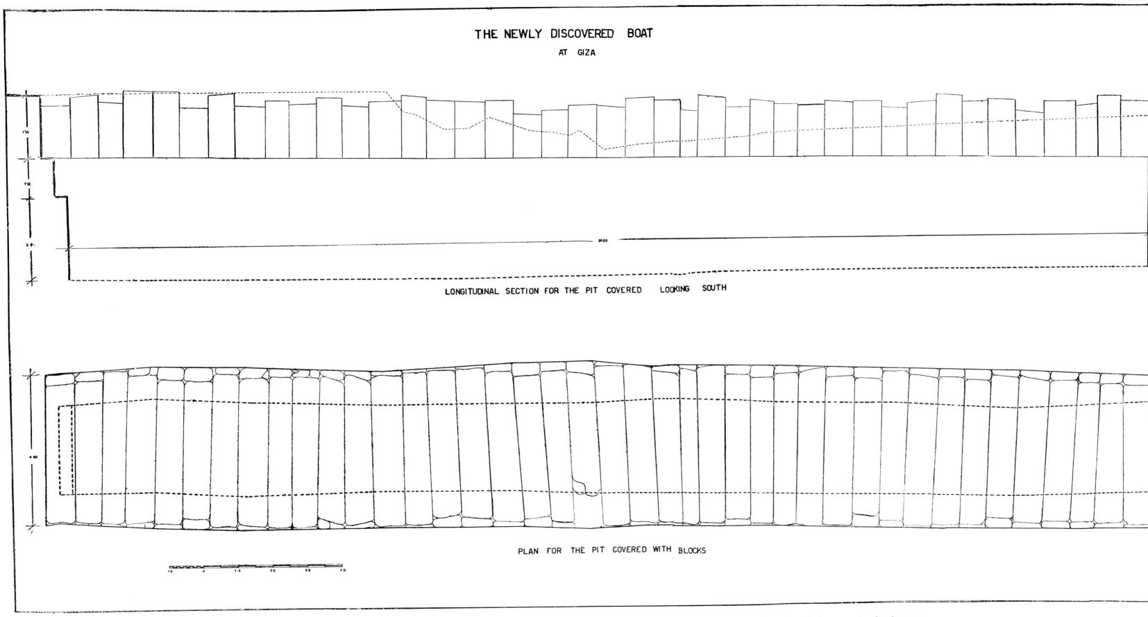
Longitudinal section for the pit covered with the blocks looking south and plan for the pit covered. In both the section and plan appear the five keystones. The small stone shutters at the extrémities of each block appear in the plan.
