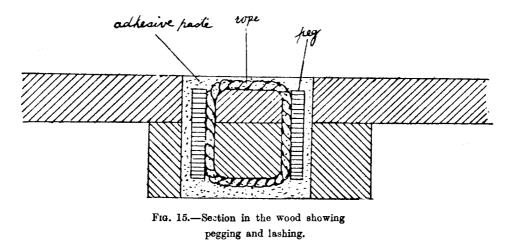
(b) *Pegging and Lashing.*—In most of the cases of pegging made in the boat, two pairs of holes were made in the two pieces to be joined, a groove was carved in the wood between the two holes, a twine run round the holes for lashing the two pieces together, a peg introduced in each of the two pairs of holes, the groove filled with the same adhesive mentioned above, and the excess paste pared away (Fig. 15).
