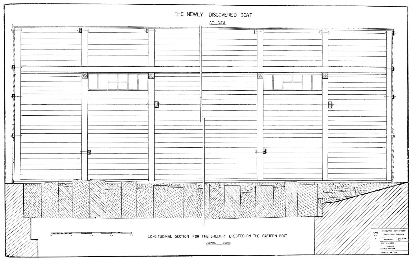
Longitudinal section for the shelter; including the pit covered with the blocks.
