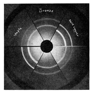
Frg. 19.—X-Ray diffraction patterns of a piece of pure copper, a piece of the staple, and a piece of brenze
