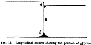
mortar used for sticking the blocks together in d and e.
