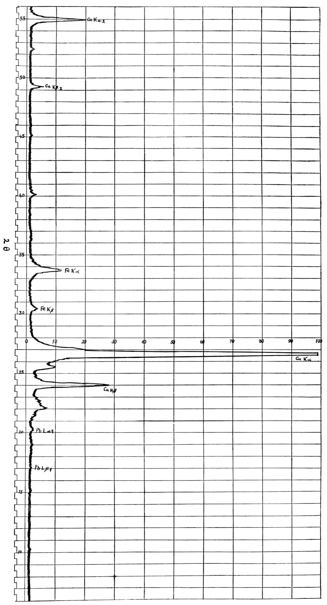
FIG. 14.-X-Ray fluorescence spectrum of small fragments of corroded copper found sticking to the sides of the limestone blocks, 50 kv, 18 m A, × 16×1,
