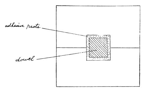
FIG. 21.-Section showing the use of flat dowels for joining adjacent wooden planks together.
